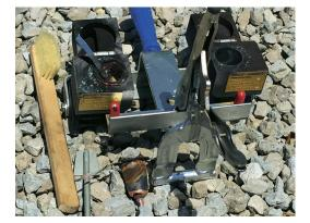
Open the mold and remove the expended steel cup - no special disposal required.
